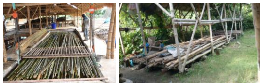
Figure 4: Treatment of bamboo is going on in tank and then under shade.
