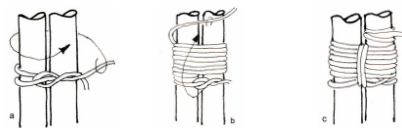
Figure 6: Shear lashing of bamboo (Schroder, 2009).
