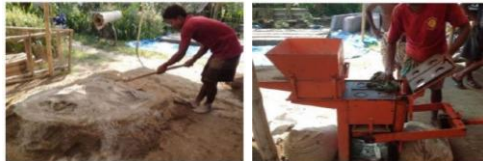
Figure 11: Mixing of mud and machine of compressed earth blocks.
