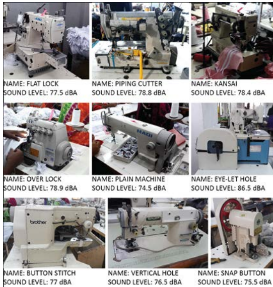
Figure 2: Nine types of machines (with sound pressure level from 1m horizontal distance) that are frequently used in the sewing section of the surveyed RMG
