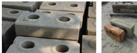
Figure 12: Size of CEB and regular brick.
